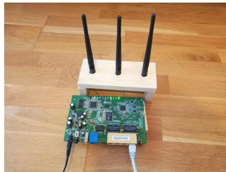
Figure 1: A WR2543ND router with the antenna array
